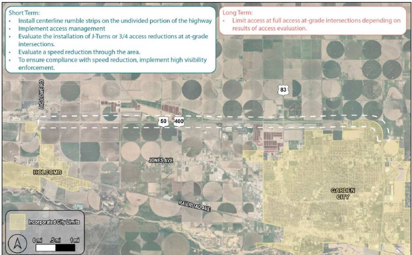
Figure 2 - U.S. 83/U.S. 50 from Big Lowe Road to Garden City Limits. Taken from Finney County Action Plan (prepared by Kimley-Horn)
