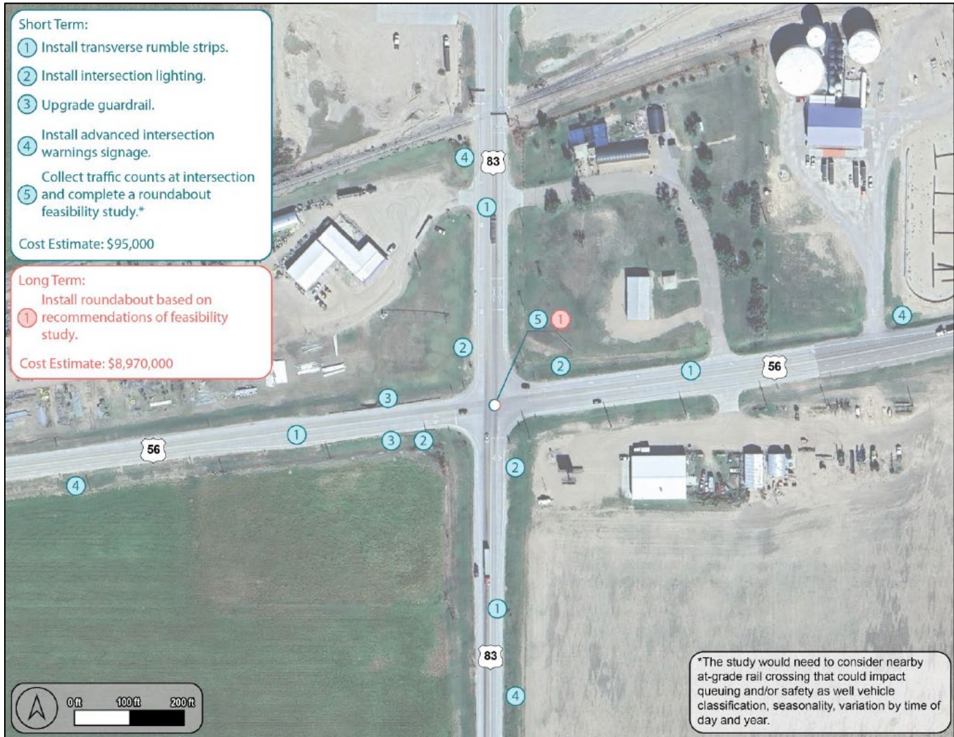
Figure 6 - Intersection of US-83 and US-56. Found in Haskell County Action Plan (prepared by Kimley-Horn).
